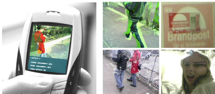
Figure 3. a) Context camera implemented on a camera phone. b) Visual effects (top-left) Effect 1: colour shadows. (top-right) Effect 2: Zoom, (bottom-left) Effect 3: Pixel, (bottom-right) Effect 4: Waves.
