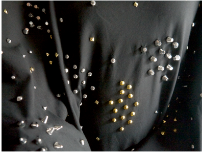
Figure 3: When an active stud touches another in a receptive cluster, an electrical connection is made, alerting the electronics that the garment is moving.
