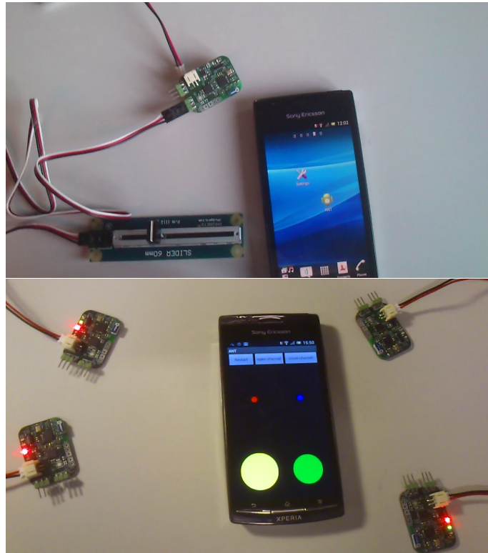
Figure 4.9: Top: Early prototyping tool working with Phidgets. Bottom: Gold Rush Inspirational Bit running in a mobile phone and custom made wireless boards.
