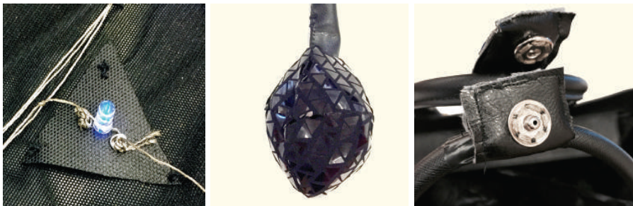
Figure 5.12: Left: LED with conductive thread. Center: Squeeze ball from resistive yarn. Right: Snap fastener switch.
