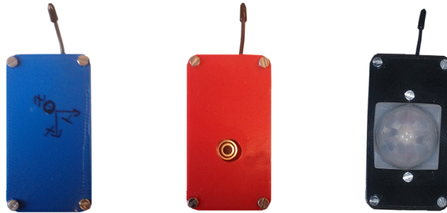
Figure 4.12: Left: Accelerometer. Center: Infrared temperature sensor. Right: presence sensor.
