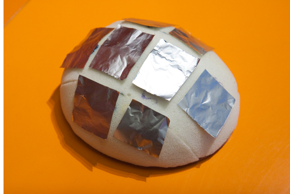
Figure 4.3: Bottom shell with the foil as electrodes for the touch sensors.
