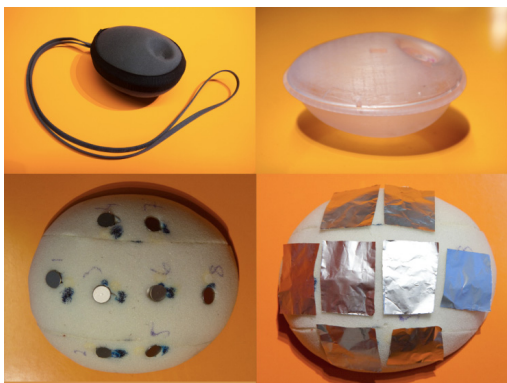
Figure 2. An assembled Lega, the inner shell, vibrator placement, and touch sensor placement.
